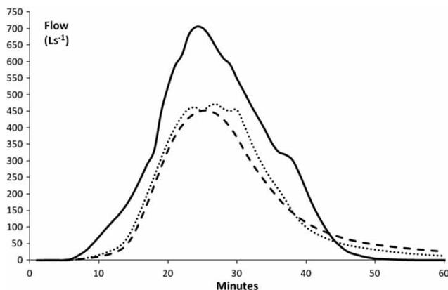
**Figure 6** | Comparison of the impacts of conventional drainage (-), SUDS management train with (-) and without green roofs (...) on outflow at Prior Deram Park, Canley, Coventry.
