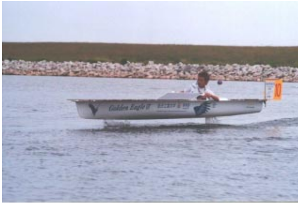
Fig. 2 The highest technology and performance has been demonstrated in Japan's Kanazawa Institute of Technology (KIT) boat, shown here in 1999 "flying" on the hydrofoils it used in both Sprint and Endurance races. KIT has won the World Championship all 3 times it has attended ('94,'97,'99); however, other boats are approaching and beating KIT performance in several events.
