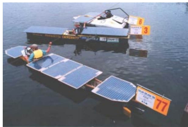
Fig. 1 Three of the 1999 boats line up for the Endurance race. Note the variation in design, with the top boat optimized for the Sprint race and the bottom boat for the Endurance race. However, all boats must compete in all events, thus the “compromise” hull of the middle boat.
