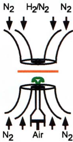
Figure 2. Experimental Setup (Red=Flame, Green=Vortex).
