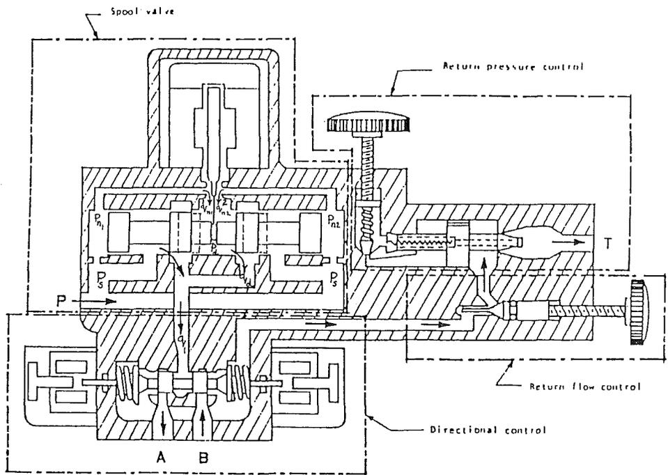
Fig. 16 Single block new servo-valve configuration
