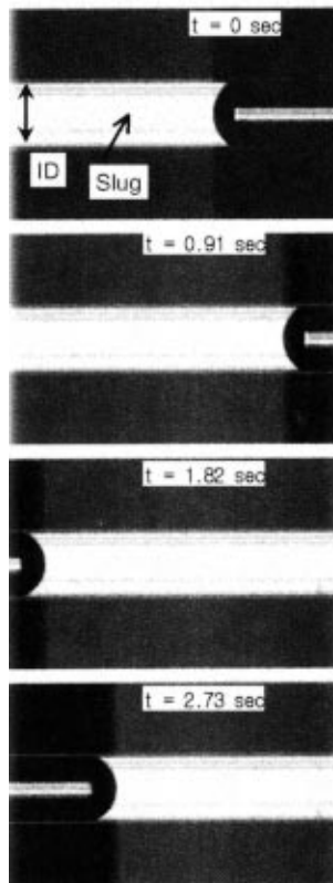
Slug Flow at \frac{Re_{gas}}{Re_{liquid}} = 9.25 (b)
