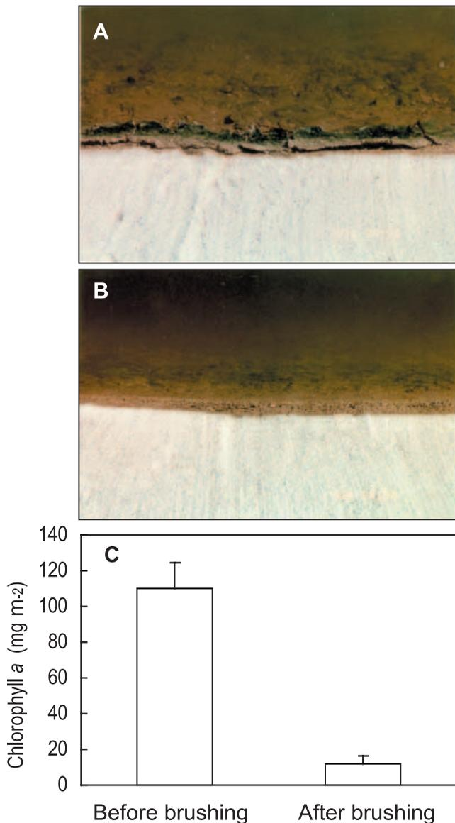
**Figure 5** | Close-up photographs of the canal wall with attached algal mat before (A) and after brushing (B). Comparison of periphyton biomass, as indicated by chlorophyll *a* concentration, before and after brushing (C).
