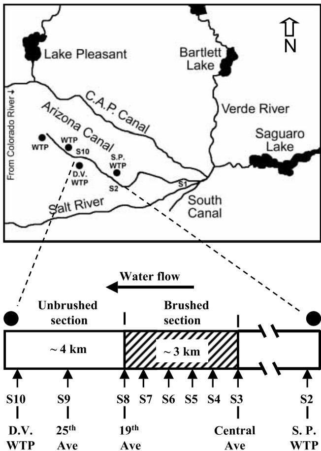
**Figure 1** | Schematic of the Arizona Canal illustrating location of water treatment plants (WTP), the brushed and unbrushed canal stretches, and sampling sites along the canal. Black circles: water treatment plants; hatched bar: brushed section (c. 3 km, between Central Avenue and 19th Avenue); open bar: unbrushed sections (c. 4 km, between 19th Avenue and Deer Valley WTP); arrows: sampling sites (S2 through S10 on the Arizona Canal).
