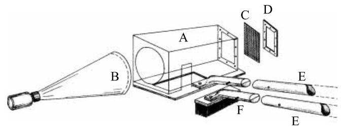
**Figure 2** | Diagram of the periphyton sampler. Sampler consists of A, a rectangular chamber with an open window (10 × 15 cm) on the bottom plate; B, a plankton net; C, a plastic screen with metal frame; D, E, two telescoping poles; and F, a wire pool brush.
