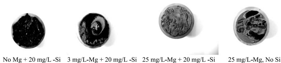
**Figure 11** | Iron scale at different magnesium levels with/without silica.
