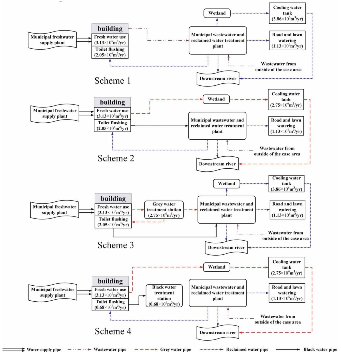
Figure 2 | Structures and water flows of the four schemes.
