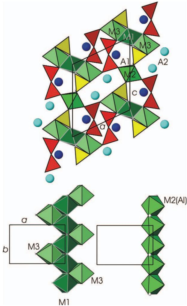
Fig. 1, Top: Polyhedral model of the clinozoisite structure (space group  $P2_1/m$ ) projected along the *b*-axis.  $\text{TO}_4$  tetrahedra are in yellow,  $\text{T}_2\text{O}_7$  groups are in red, octahedra in green, A sites are shown as blue spheres (A1 dark blue, A2 light blue); Bottom: Linkage of octahedral sites forming chains parallel to the *b*-axis. H atoms on the chain formed by M2 octahedra are shown as small white spheres.
