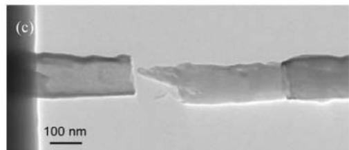
Figure 2 (a) Load-elongation measurements for MWCNTs tested under various irradiation conditions. (b) Typical fracture of a MWCNT subjected to ion beam irradiation showing failure
