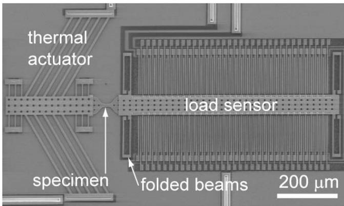
Figure 1 The n-MTS consists of a thermal actuator which provides displacement-controlled loading and a differential capacitive sensor to detect the corresponding load. The
