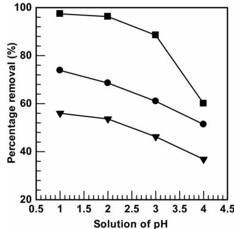
**Figure 8** | Effect of solution of pH on regeneration of  $\text{Cr}^{+3}$  (●),  $\text{Cd}^{+2}$  (■) and  $\text{Zn}^{+2}$  (▼) ion sorbed on *A. pinnata* powder shell.
