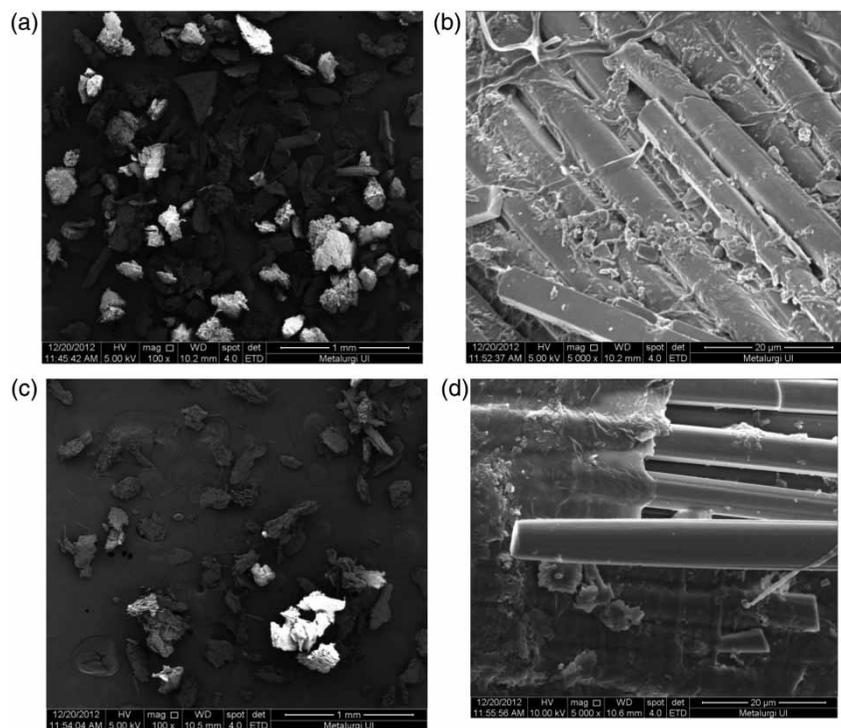
**Figure 3** | Scanning electron image of *A. pinnata* sample at the following magnifications: (a) 100 $\times$ , (b) 5,000 $\times$ , (c) after loaded Cr 100 $\times$ , (d) after loaded Cr 5,000 $\times$ . Scale as indicated in photo.
