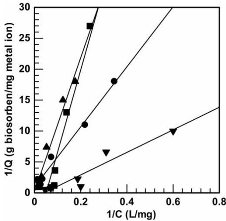
**Figure 7** | Langmuir isotherm for biosorption of  $\text{Cr}^{+3}$  (●),  $\text{Cr}^{+6}$  (▲),  $\text{Cd}^{+2}$  (■) and  $\text{Zn}^{+2}$  (▼) by *A. pinnata* powder shell.
