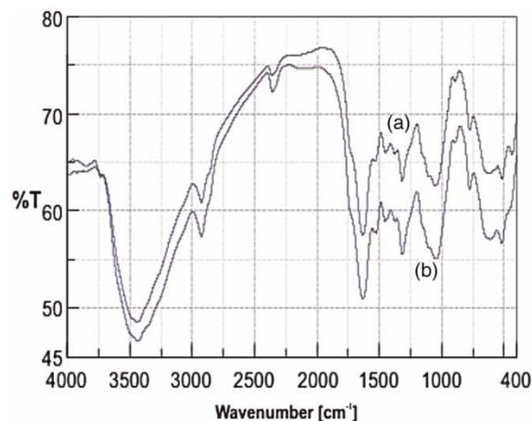
Figure 2 | FTIR spectrum of *A. pinnata* shell powder before (a) and after (b) sorption of Cr(III).
