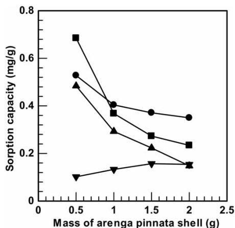
**Figure 5** | Effect of mass of *A. pinnata* powder shell on sorption capacity of Cr<sup>+3</sup> (●), Cr<sup>+6</sup> (▲), Cd<sup>+2</sup> (■) and Zn<sup>+2</sup> (▼).
