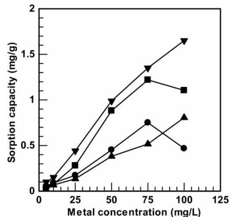
**Figure 6** | Effect of concentration of Cr<sup>+3</sup> (●), Cr<sup>+6</sup> (▲), Cd<sup>+2</sup> (■) and Zn<sup>+2</sup> (▼) solution on sorption capacity by *A. pinnata* powder shell.
