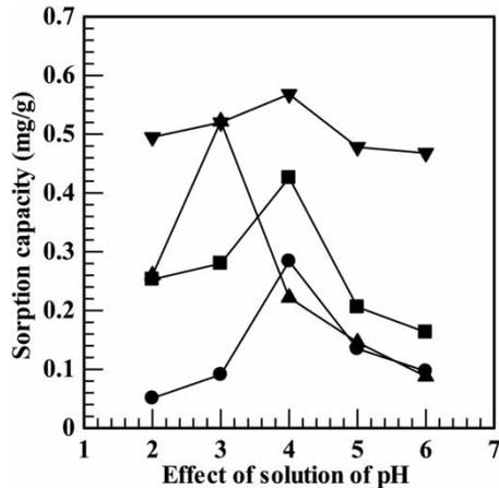
**Figure 4** | Effect of solution of pH on sorption capacity of Cr<sup>+3</sup> (●), Cr<sup>+6</sup> (▲), Cd<sup>+2</sup> (■) and Zn<sup>+2</sup> (▼).
