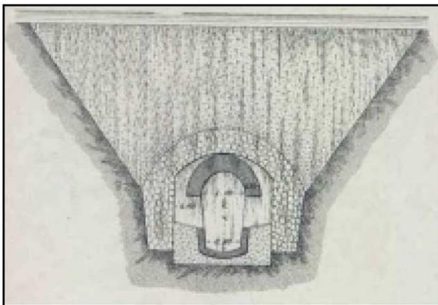
Figure 3 | Drawing of filtering tunnel (Zannoni 1868).
