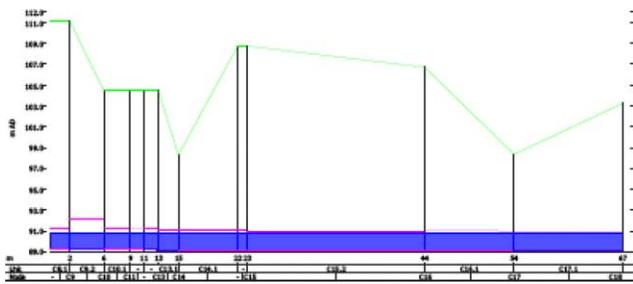
**Figure 7** | Hydraulic profile of tunnel corresponding to Bocca Rio Conco ( $Q = 0.558 \text{ m}^3/\text{s}$ ).
