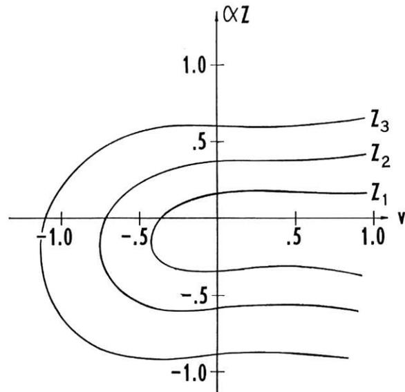
Fig. 17 Pump-turbine data with transformed ordinate speed  $\times$  gate ( $\alpha z$ )
