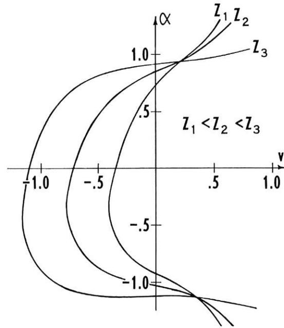
Fig. 16 Flow/speed representation of pump-turbine data for variable gate ( $z$ ) at unity head
