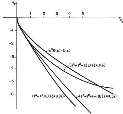
Fig. 8 Projections into the  $e_1e_2$  plane of zero-trajectories of four systems
