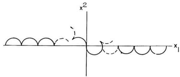
Fig. 7 Sketch of optimum switching curve in  $x^1x^2$ -plane for  $\zeta \rightarrow 0$  and  $\gamma \gg 0$
