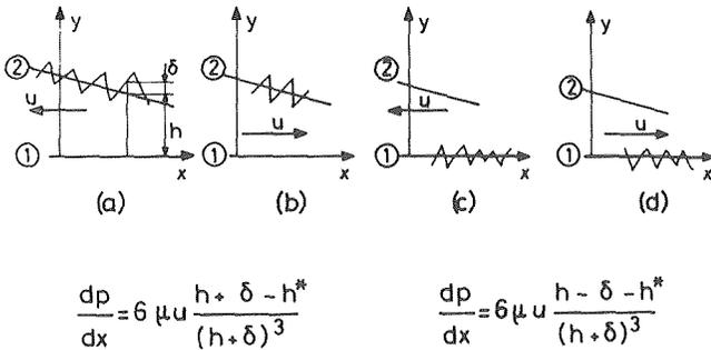
Fig. 4 The hydrodynamics of a slider
