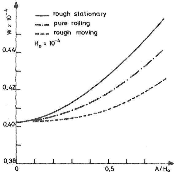
Fig. 3 Load capacity versus roughness ratio (transverse roughness) for two rotating cylinders
