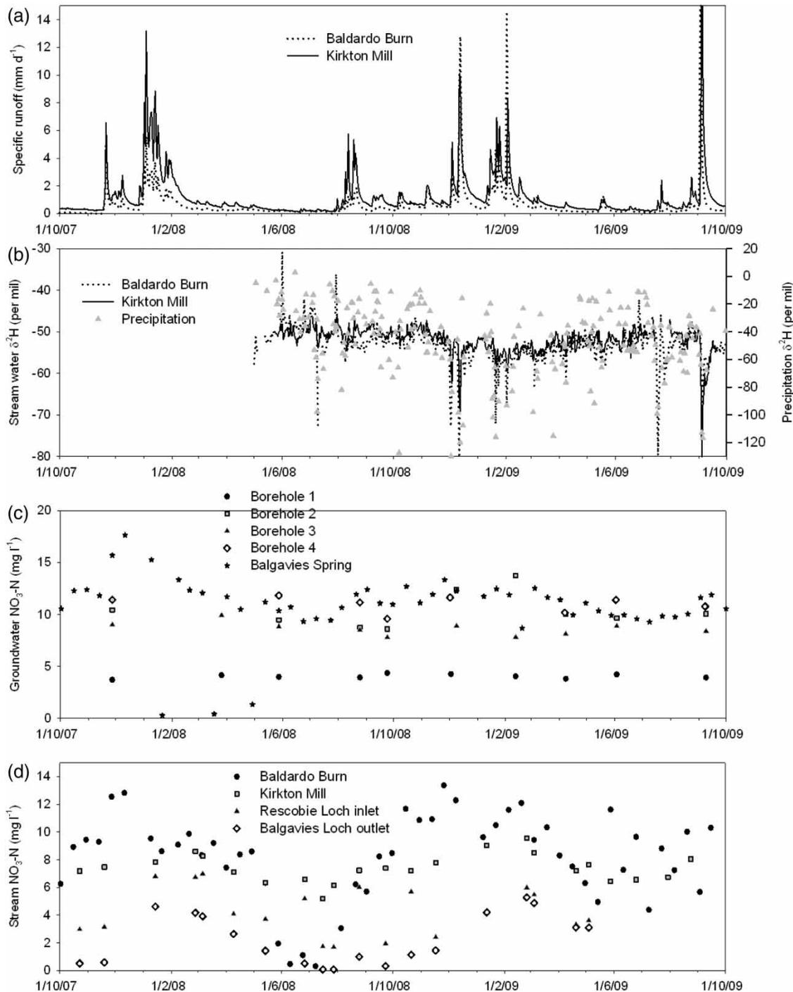
**Figure 4** | Monitoring data from the Lunan catchment including (a) specific discharge, (b) daily  $\delta^2\text{H}$  measurements from precipitation and stream water, (c) groundwater nitrate concentrations and (d) stream nitrate concentrations.
