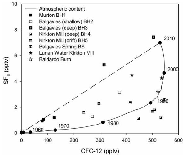
**Figure 2** | CFC-12 and SF<sub>6</sub> for each sample plotted together with a curve depicting the time-course relationship of atmospheric CFC-12 to SF<sub>6</sub>. The dashed line represents simple mixing between modern and pre-1950s water.
