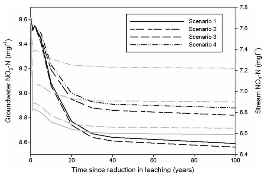
**Figure 7** | Time-course of reduction in nitrate concentrations for groundwater (black lines) and stream water (grey lines) according to various management scenarios, based on a groundwater mean solute transit time of 30 years.
