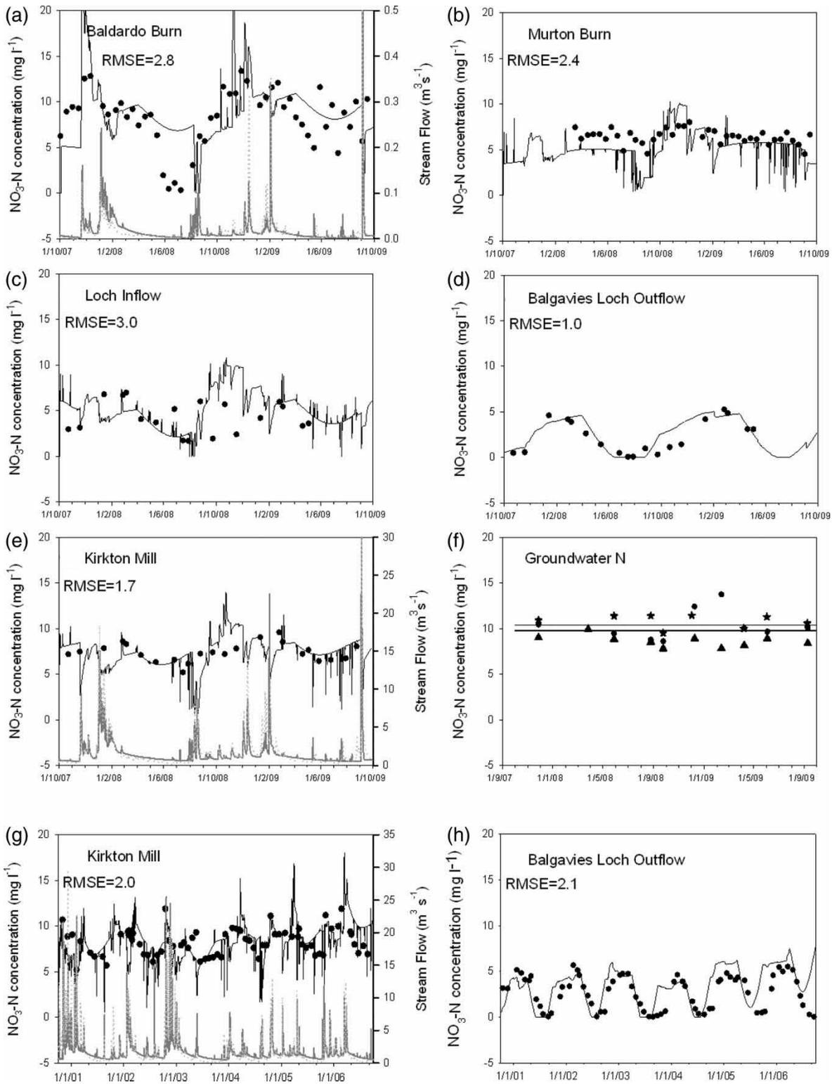
**Figure 6** | Results of model calibration simulations for Oct 2007–Oct 2009 at 5 stream sites (a)–(e) and for groundwater recharge (f), and model validation simulations for Oct 2000–Oct 2006 at two stream sites (g) and (h).
