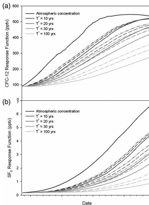
**Figure 3** | Groundwater response functions for (a) CFC-12 and (b) SF<sub>6</sub> obtained by applying a range of dispersion models to historic concentrations of the atmospheric trace gases. Solid lines represent results with  $P_D^*=0.3$ , dashed lines  $P_D^*=0.5$  and dotted-dashed lines  $P_D^*=0.7$ .
