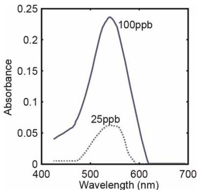
**Figure 4** | Measured absorbance at various wavelengths for 25 and 100 ppb chromium (VI) concentrations.
