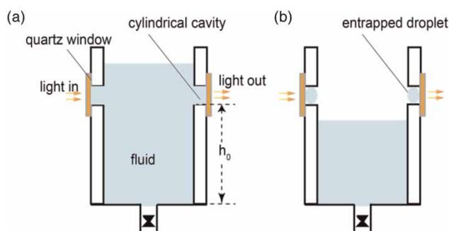
**Figure 2** | As the cell is being filled, the liquid also occupies the cavities. On emptying the cell, liquid droplets are entrapped in the cavities.
