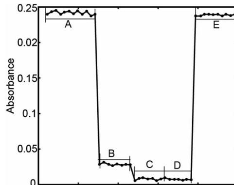
Figure 8 | The reversibility of the signal response after cell rinsing. A is absorbance for 100 ppb chromium (VI), B, C, and D are the absorbance after first, second, and third cell rinsing, respectively. E is the absorbance on subsequent testing of an aliquot of 100 ppb chromium (VI).
