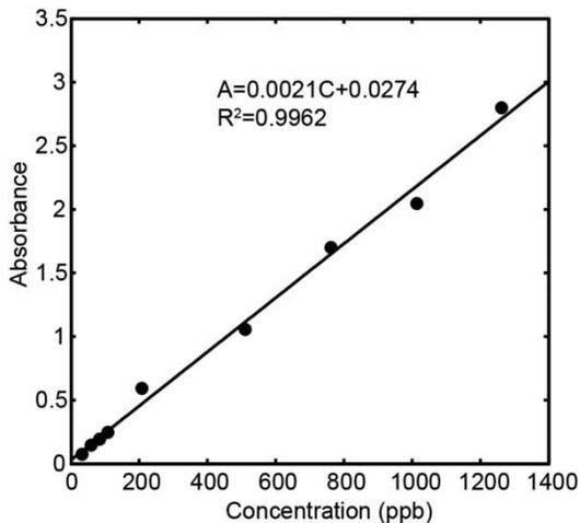
Figure 7 | Chromium (VI) calibration over a range of 25 to 1,250 ppb.
