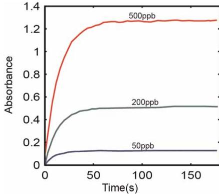
Figure 5 | Time response of reaction between chromium (VI) sample and reagent.
