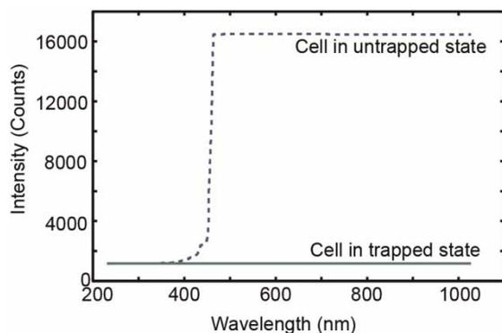
**Figure 3** | Received light intensity spectrum (counts) for when the cell is in the 'trapped' and 'untrapped' states.
