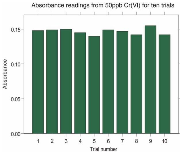
Figure 6 | Measured absorbance for ten tests with 50 ppb chromium (VI).
