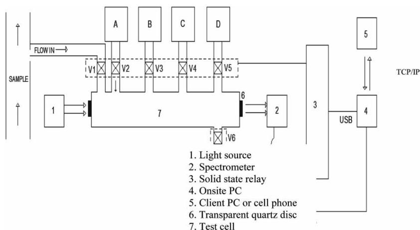
**Figure 1** | Components of proposed discrete analyzer (not drawn to scale). A, B, C, and D are for reagent, standard, and deionized water.
