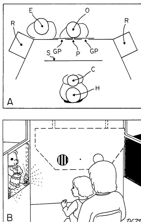
**Fig. 1.** Schematic drawings of OPL apparatus with animal reinforcers. **A**, Top view. *H*, Holder (parent); *C*, child; *S*, holder's shield; *R*, plexiglass box containing toy animal reinforcer; *E*, experimenter; *O*, observer; *P*, peephole; *GP*, grating position. **B**, Frontal view. Toy animals were illuminated and visible only when activated; otherwise a covering of darkened plexiglass obscured them from view. Dashed lines indicate position of holder's eye shield.
