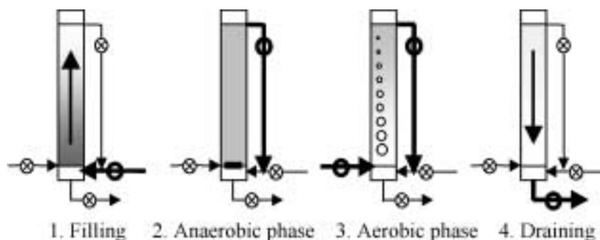
**Figure 1** Operating sequence for the SBBR
