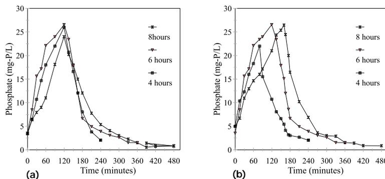
**Figure 3** The profiles of phosphate level of bulk solution over cycle duration in different HRTs with the same anaerobic time of two hours (a), and with the same An/Ox time ratio of 1:2 (b)
