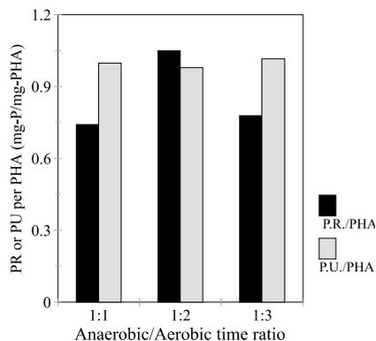
**Figure 6** The P release and uptake level per PHA at various An/Ox time ratios
