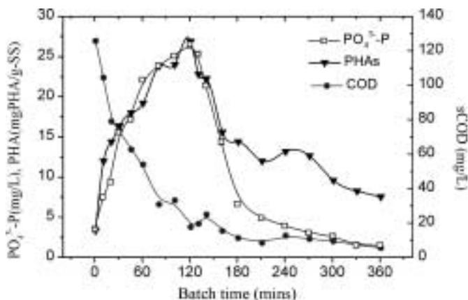
**Figure 2** PO<sub>4</sub>-P, PHA and sCOD concentration profiles through batch time with HRT
