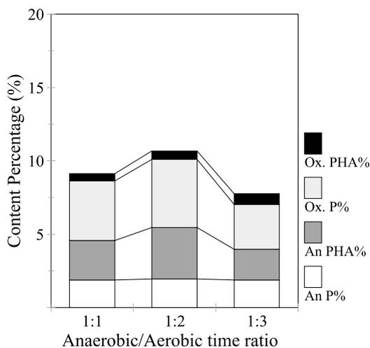
**Figure 5** The PHA and P content of the biofilm at different An/Ox time ratios
