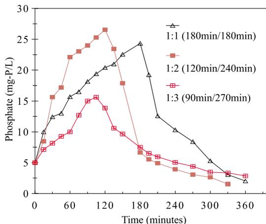
**Figure 4** The phosphate level in the bulk solution at different An/Ox time ratios
