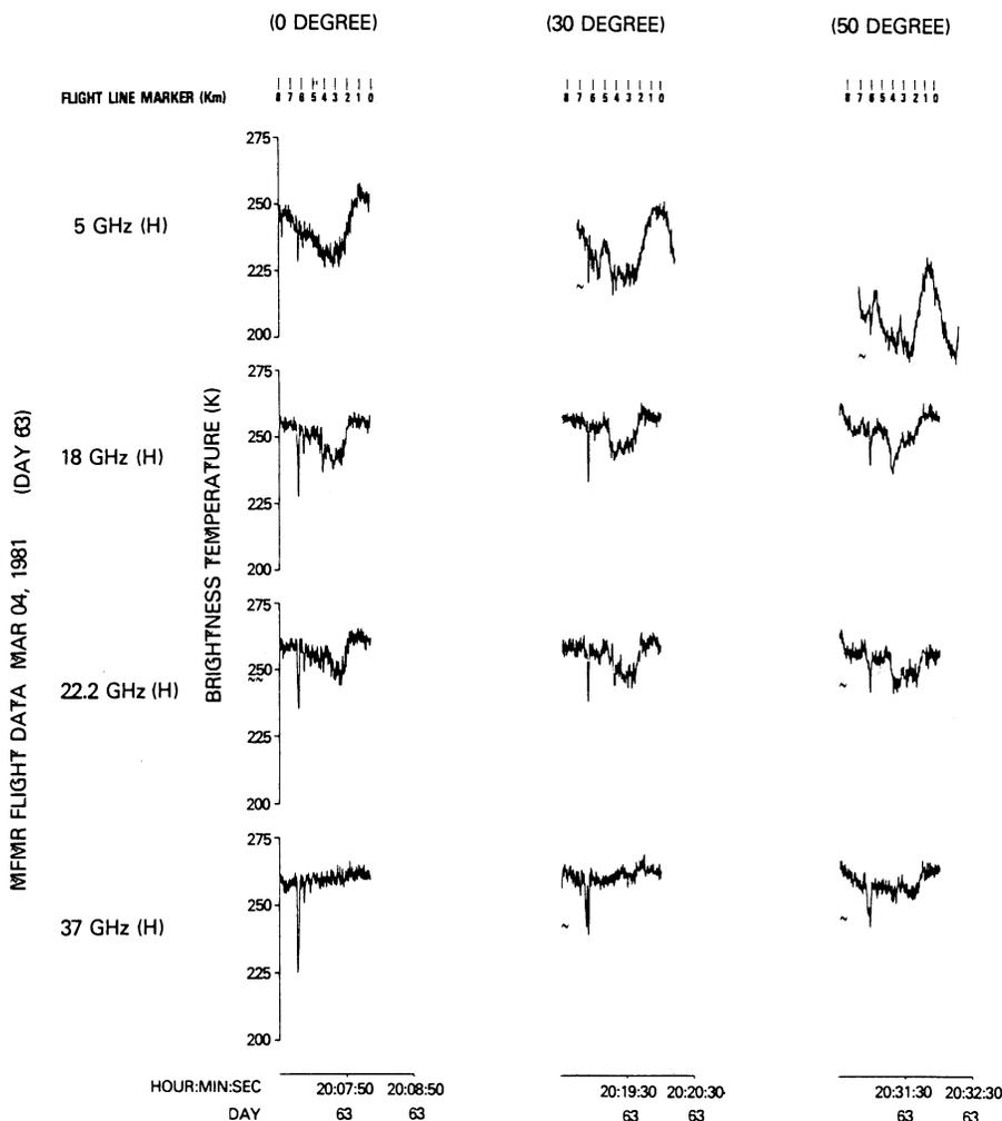
Fig. 2. Horizontally polarized microwave brightness temperatures along the flight line for 5 GHz (C Band), 18 GHz (Ku Band), 22.2 GHz (K Band) and 37 GHz ( $K_A$  Band) at  $0^\circ$ ,  $30^\circ$  and  $50^\circ$  incidence angles.
