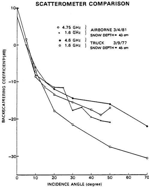
Fig. 4. Comparison of scatterometer returns obtained by aircraft sensors and the truck system.
