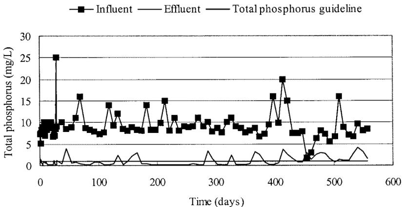
Figure 2 Phosphorus removal (results from the 8 day test controls)
