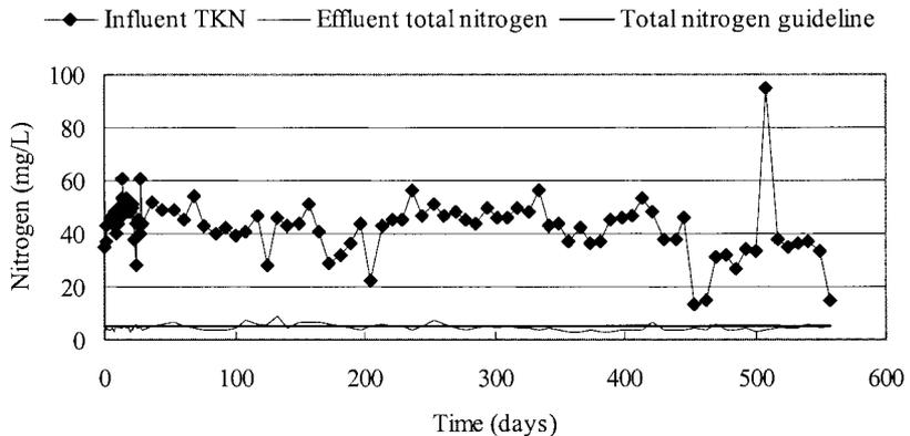
Figure 1 Nitrogen removal (results from the 8 day test controls)
