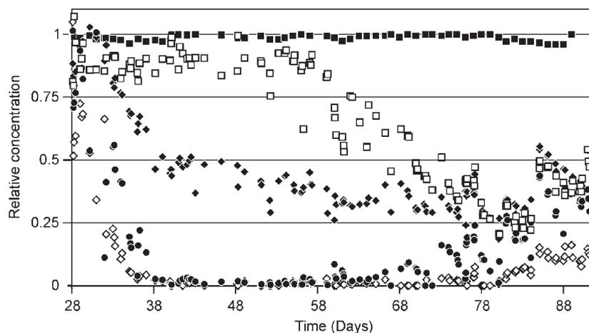
**Figure 4** Relative concentrations of indole (●), quinoline (◇), benzothiophene (◆), dibenzofuran (□), and chloride (■) as a function of time from day 28 to 92
