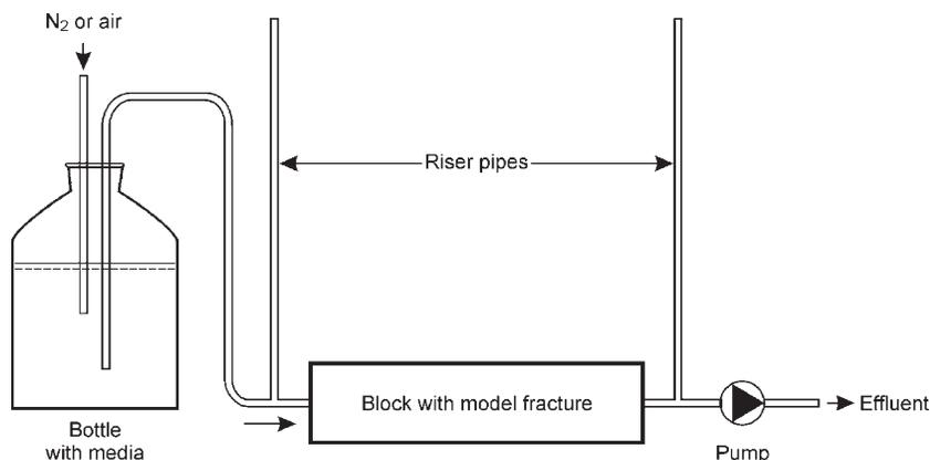
**Figure 2** The experimental set-up
