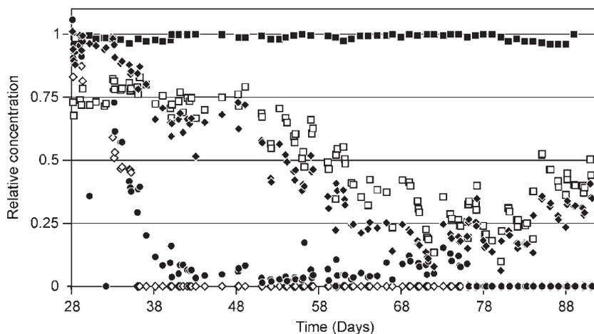
**Figure 3** Relative concentrations of phenol (◇), o-cresol (●), 2,4-dimethylphenol (□), 3,5-dimethylphenol (◆), and chloride (■) as a function of time from day 28 to 92
