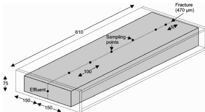
**Figure 1** The flow model. All the numbers are in mm except where noted in the figure
