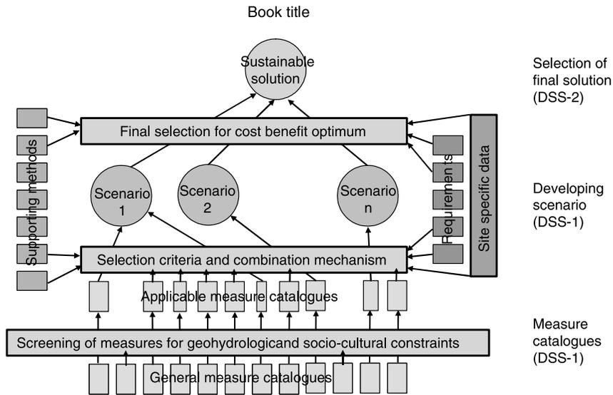
**Figure 3** Structure of the two stage Decision Support System
