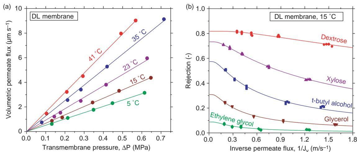
**Figure 1** | Experimental measurements of DL membrane–neutral solutes phenomenological parameters. Pure water permeabilities at various temperatures are depicted in (a). Neutral solutes reflection coefficients and diffusive permeabilities are estimated from (b).
