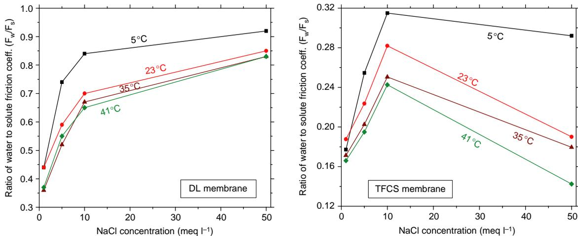
Figure 6 | Effects of concentration and temperature on  $F_w/F_s$  for NaCl.
