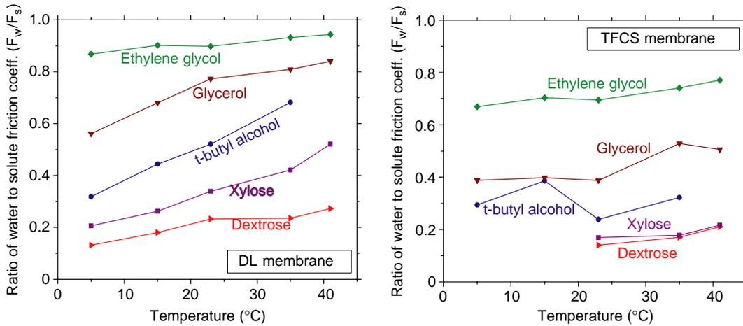
Figure 4 | Temperature effects on the ratio of the total friction to water transport to the total friction to solute transport for both membranes.
