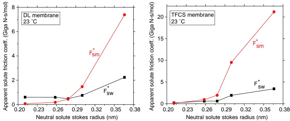
**Figure 2** | Friction coefficients for neutral solute–membrane and neutral solute–water interactions for both membranes at room temperature.
