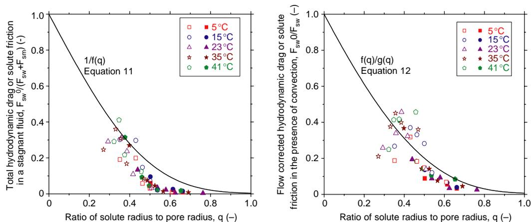
**Figure 5** | Comparison of frictional coefficient ratios with hydrodynamic models of hindered transport. Open symbols represent DL membrane data and filled symbols correspond to the TFCS membrane.
