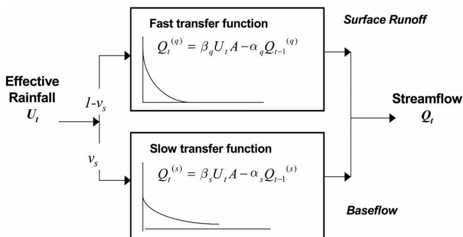
Figure 3 | IHACRES linear routing model structure.
