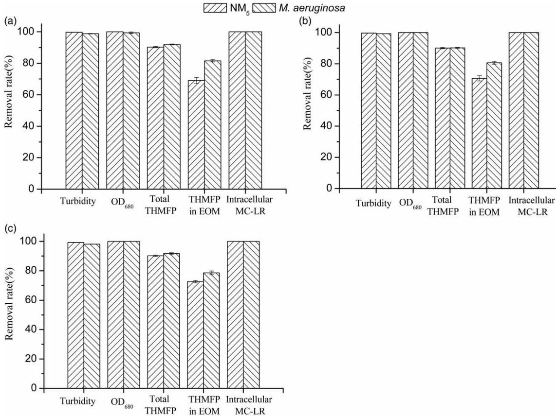
**Figure 2** | Results of coagulation-sedimentation of *M. aeruginosa* solution and a mixture of NB and *M. aeruginosa* after a 5-day incubation (*NM<sub>5</sub>*). Coagulant: (a) Al<sub>2</sub>(SO<sub>4</sub>)<sub>3</sub> 20 mg Al<sub>2</sub>O<sub>3</sub>/L; (b) FeCl<sub>3</sub> 44.5 mg Fe<sub>2</sub>O<sub>3</sub>/L; (c) PAC 39 mg Al<sub>2</sub>O<sub>3</sub>/L.
