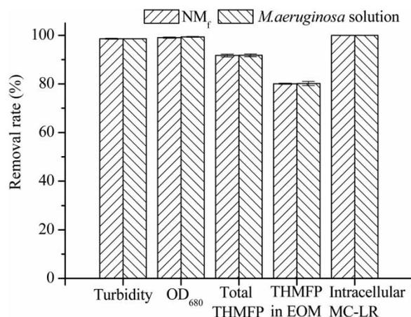
**Figure 1** | Results of coagulation-sedimentation of *M. aeruginosa* solution and the fresh mixture of NB and *M. aeruginosa* without incubation ( $NM_f$ ). Coagulant:  $Al_2(SO_4)_3$  at the optimized dosage of 20 mg  $Al_2O_3/L$ ;  $25 \pm 1$  °C.
