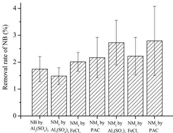
**Figure 3** | Removal of NB by coagulation-sedimentation with three types of coagulants. Coagulant dosage: Al<sub>2</sub>(SO<sub>4</sub>)<sub>3</sub> 20 mg Al<sub>2</sub>O<sub>3</sub>/L; FeCl<sub>3</sub> 44.5 mg Fe<sub>2</sub>O<sub>3</sub>/L; PAC 39 mg Al<sub>2</sub>O<sub>3</sub>/L. *NM<sub>5</sub>* – a mixture of NB and *M. aeruginosa* after a 5-day incubation. *NM<sub>f</sub>* – a fresh mixture of NB and *M. aeruginosa* without incubation.
