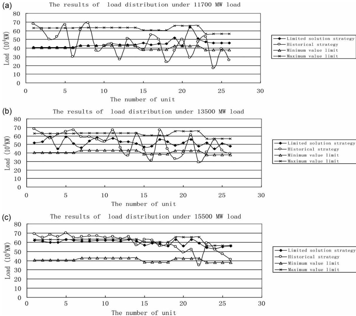
**Figure 5** | The comparison between the two algorithms for optimal load distribution under three three-level magnitude loads corresponding to a 74 m water head.
