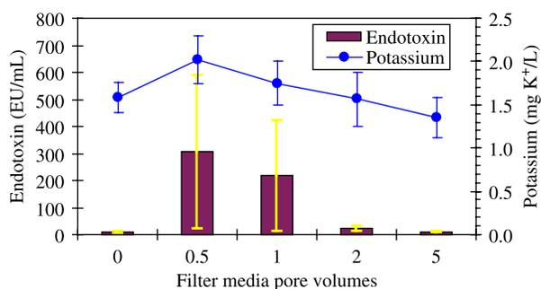
**Figure 5** | Average endotoxin and potassium concentrations vs. pore volumes for 18 h filter shutdowns ( $n = 6$ ).
