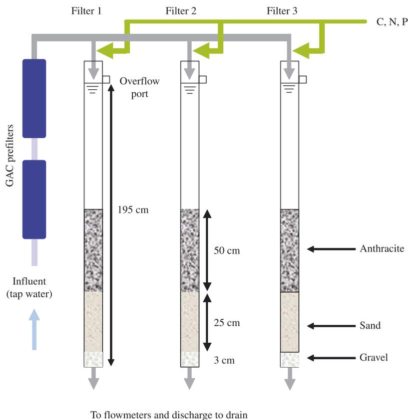
**Figure 1** | Diagrammatic representation of bench-scale filter column set-up.
