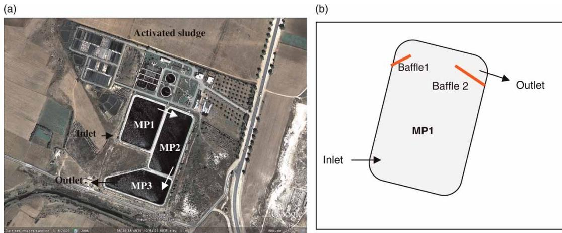
**Figure 1** | (a) Overview of Korba's wastewater treatment (36°39'38.48" N, 10°54'21.69" E; Google photo); (b) position of the baffles inside MP1.
