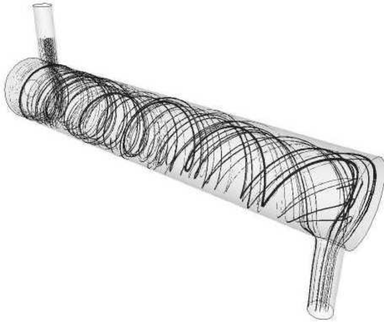
Figure 11 | Particle tracks coloured by dose for configuration 3.
