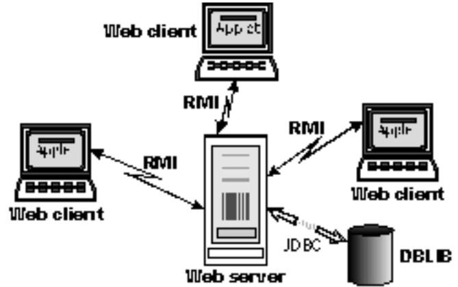
Figure 6 | Schematic representation of the basic RMI model.
