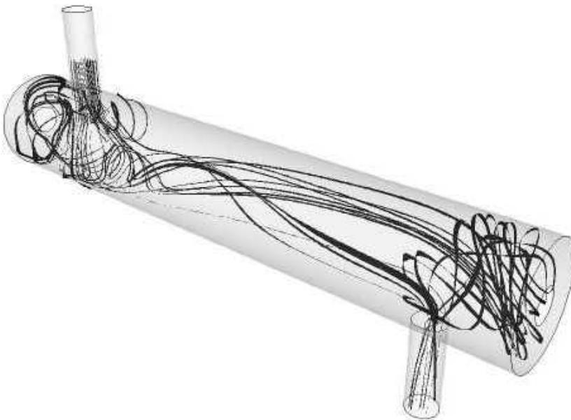
**Figure 10** | Particle tracks coloured by dose for configuration 2.
