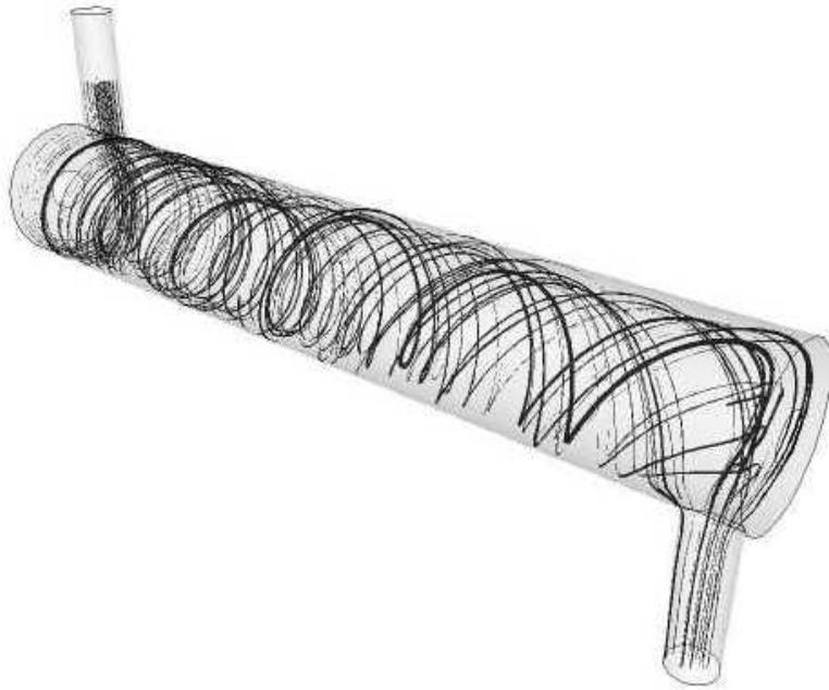
**Figure 11** | Particle tracks coloured by dose for configuration 3.
