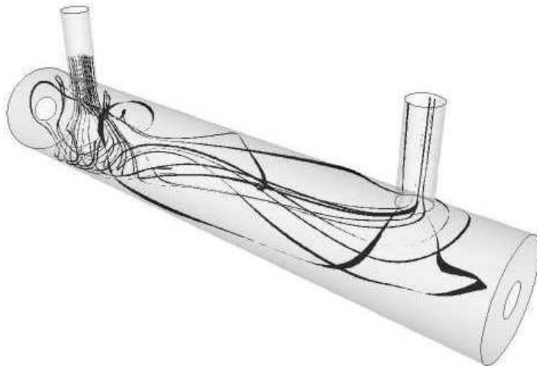
**Figure 12** | Particle tracks coloured by dose for configuration 4.
