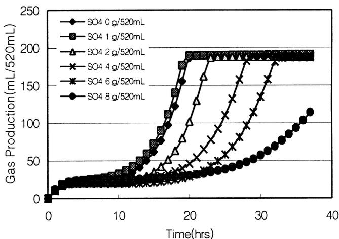
**Figure 6** Gas production profile for different sulfate concentrations
