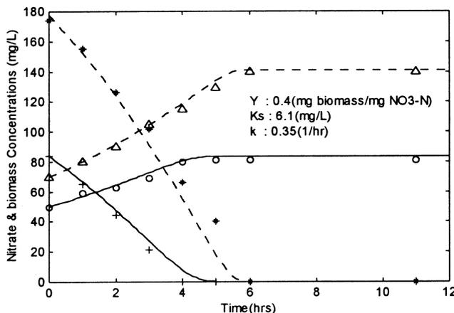
**Figure 3** Nitrate depletion and biomass growth profiles in two batch reactors (The symbols show measured data; lines show model prediction)
