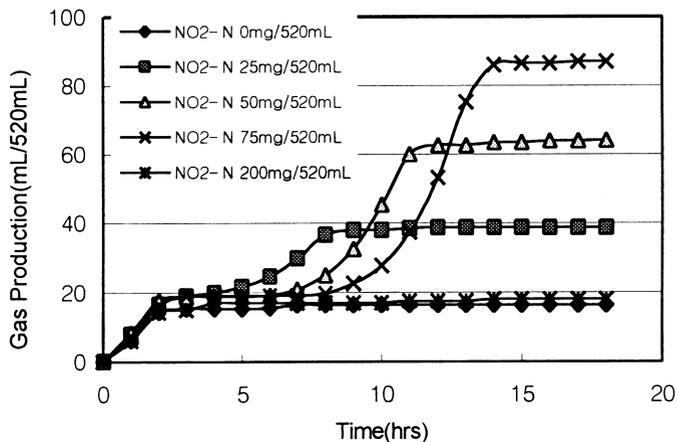
Figure 8 Gas production profile for different nitrite concentrations
