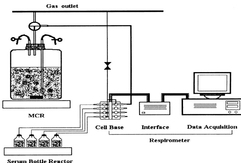
Figure 1 Schematic diagram of the MCR, batch serum bottle reactors and respirometer system
