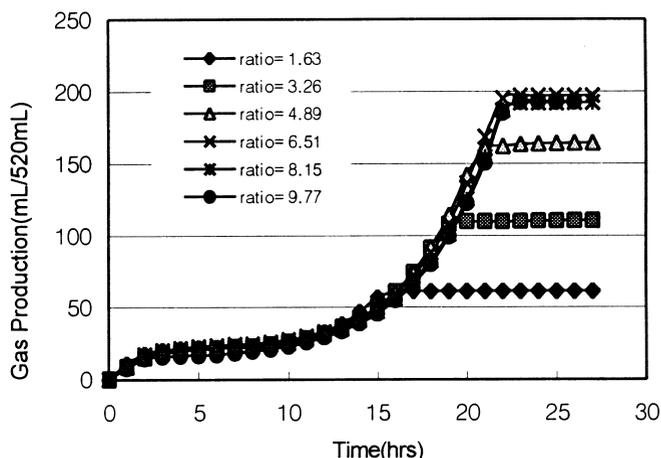
Figure 4 Gas production profile for different  $S_2O_3^{2-}/NO_3^-N$  ratios
