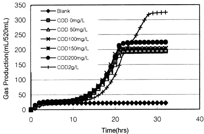
Figure 7 Gas production profile for different COD concentrations under mixotrophic conditions
