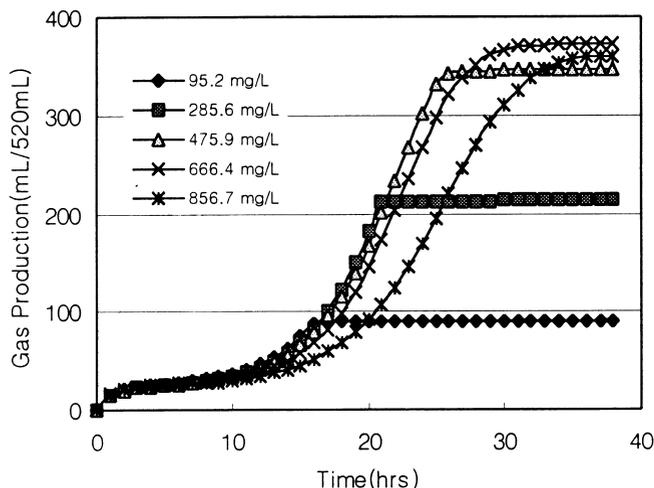
**Figure 5** Gas production profile for different  $\text{NO}_3\text{-N}$  concentrations
