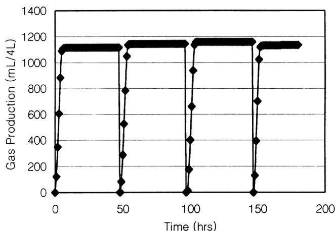
**Figure 2** Gas production during feeding cycles of the MCR
