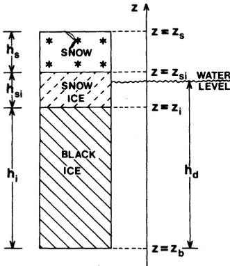
Fig. 1. Cross-section of a floating ice sheet with the vertical coordinate system.
