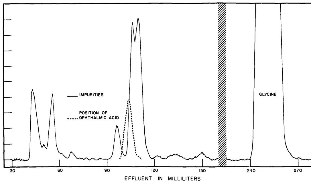
Fig. 1. A radiochromatogram of commercially obtained <sup>14</sup>C-labeled glycine showing the correspondence of the location of an impurity with ophthalmic acid. The amino acid was chromatographed on an automatic amino acid analyzer and the effluent fluid monitored continuously with a liquid flow detector for radioactivity.
