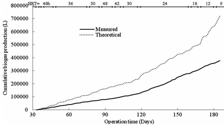
**Figure 5** | Cumulative biogas production produced by the SGBR.
