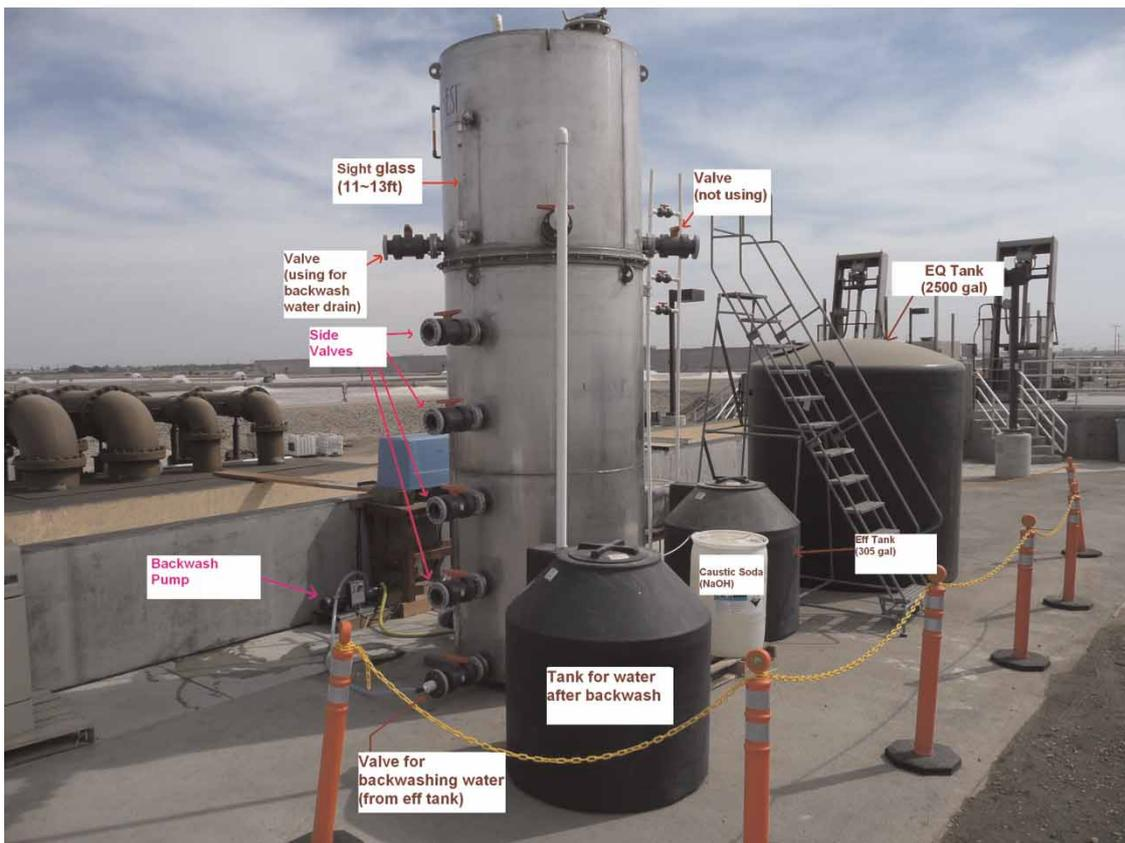
Figure 1 | Schematic of the pilot-scale SGBR system.
