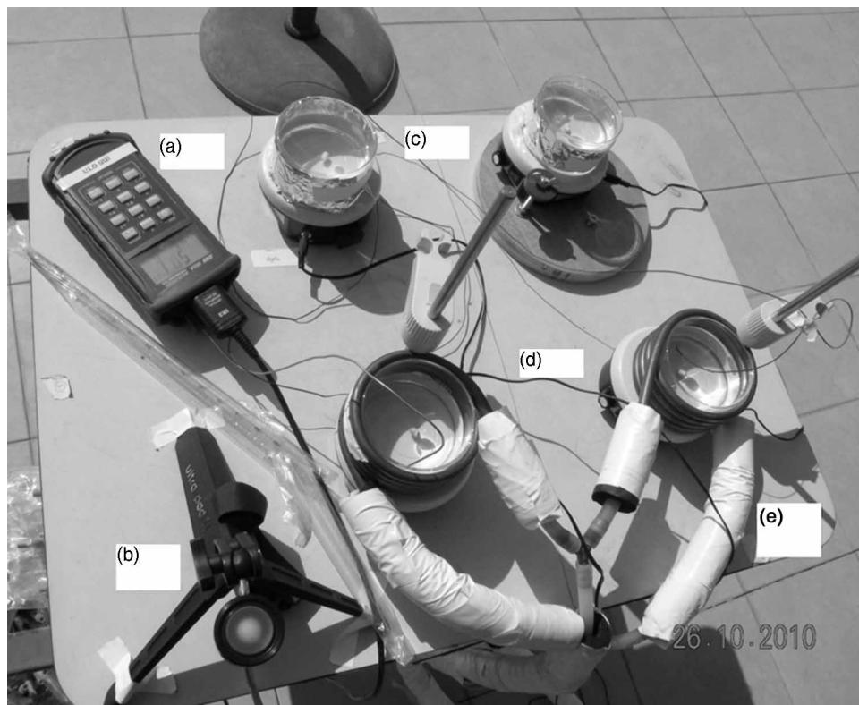
Figure 1 | Field experiment set-up: (a) thermocouple, (b) spectroradiometric detector, (c) glass dishes exposed to solar radiation only, (d) test dishes exposed to solar radiation and heat via water flowing through the copper tube, (e) insulation layer around the silicone tube that connects the copper tube to the chiller.
