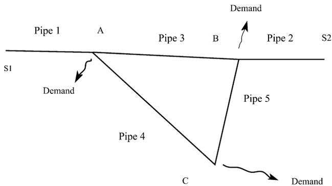
**Figure 12** | The modified delta connection, showing two sources delivering water to the delta connection, as compared with the delta connection diagram shown in Figure 10.
