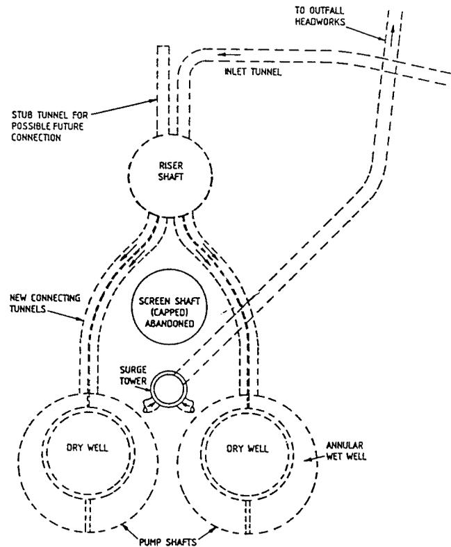
Figure 2 | Modified arrangement of Bandra IPS.
