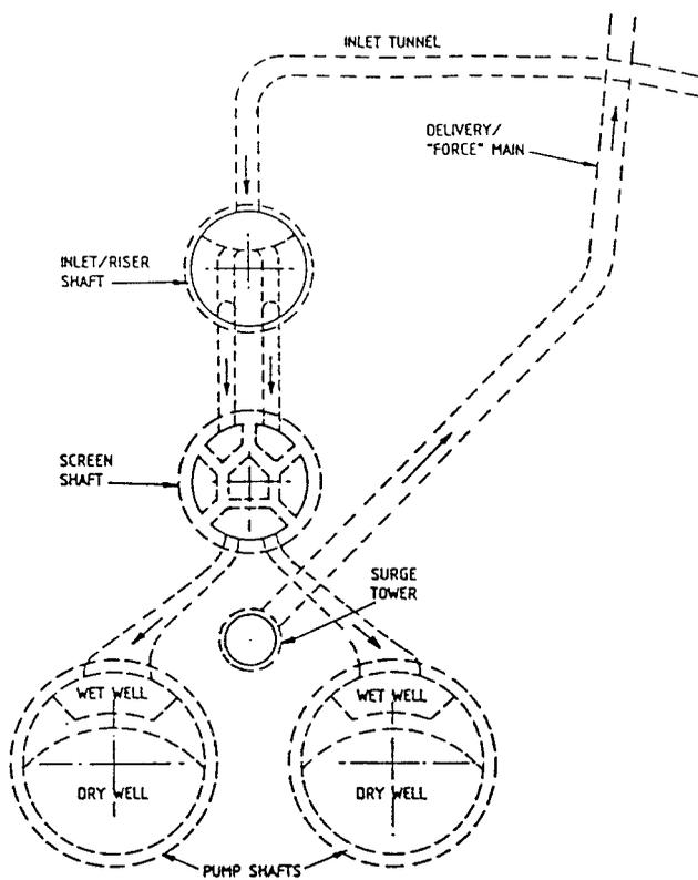
Figure 1 | Original layout of Bandra Influent Pumping Station.
