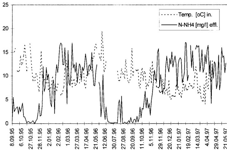
**Figure 2** Effluent ammonium concentration as a function of the influent temperature
