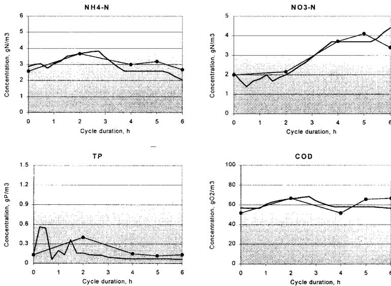
**Figure 3** Results of dynamic calibration of the model of SBR nr 2 at Nowy Targ WWTP (●: observations; —: simulation)
