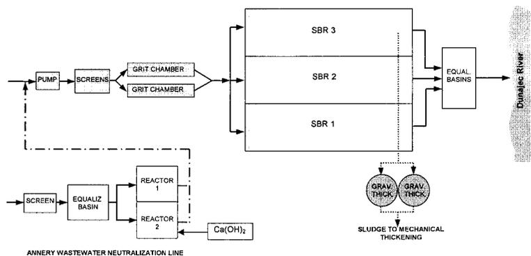
Figure 1 Layout of the Nowy Targ WWTP
