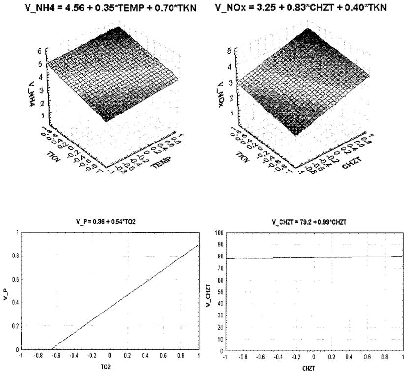
**Figure 6** Simulated relationships of removal rates for organic compounds ( $V_{ChZT}$ ), phosphorus ( $VP$ ), ammonia nitrogen ( $V_{NH4}$ ) and nitrates ( $V^{NO3}$ ) as a function of COD and TKN in influent, wastewater temperature and length of aeration phase. (Note:  $V_{ChZT} = V_{COD}$ )
