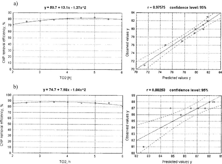
**Figure 4** Simulated relationship of CNP removal efficiency and duration of the aeration phase in SBR in Nowy Targ at wastewater temperature 6°C (a) and 14°C (b)
