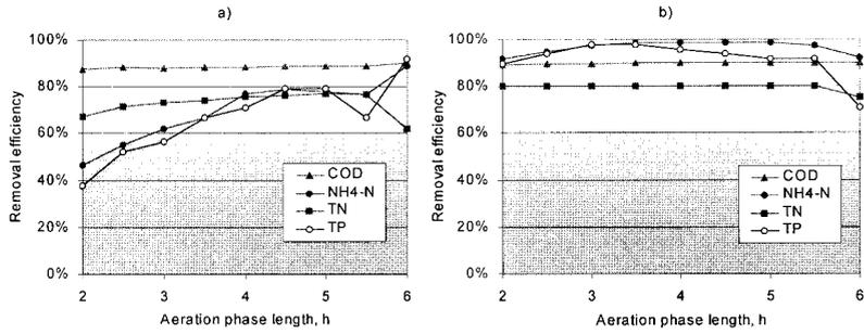
**Figure 5** Simulated removal efficiency of CNP compounds in SBR in Nowy Targ WWTP at temperature 6°C (a) and 14°C (b) as function of the aeration phase length
