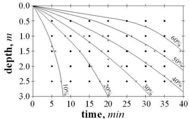
Figure 2 | Example of iso-removal curves from settling analysis.
