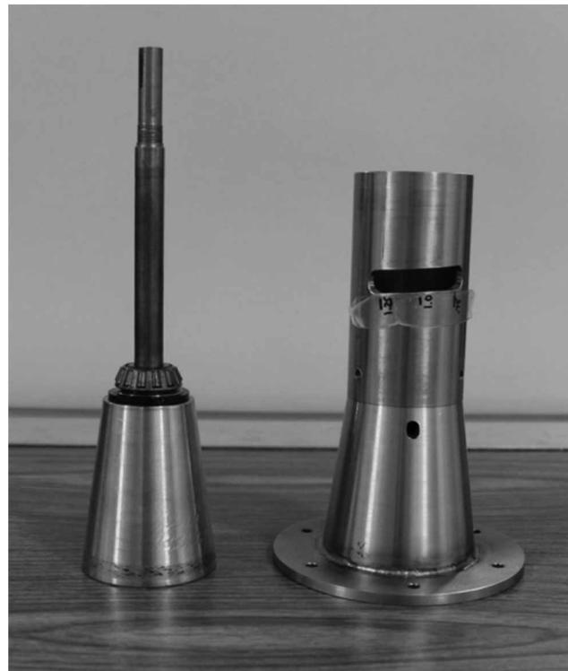
**Figure 3** | The cone (left) rotates inside the housing (right).
