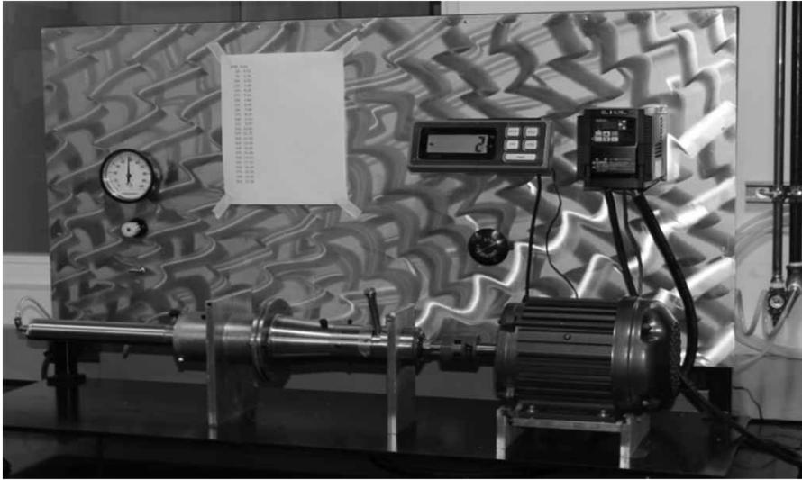
**Figure 2** | Instrumented reactor to process fecal and simulant solids.
