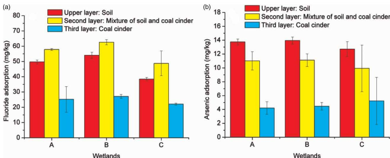
Figure 5 | Fluoride and arsenic adsorption of wetland substrates.
