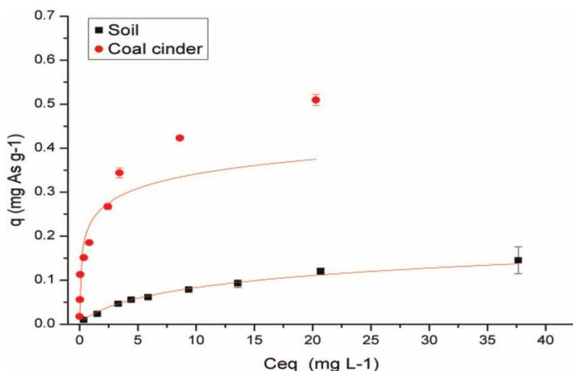
**Figure 2** | Relation between equilibrium solution As and adsorbed As for soil and coal cinder.
