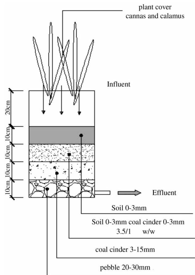
Figure 1 | Schematic diagram of semi-pilot scale vertical-flow constructed wetland.
