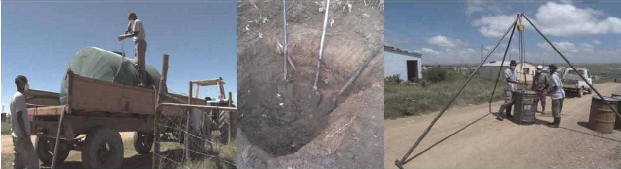
**Figure 2** | Some of the specially designed tools used by franchisees: a tractor-mounted tank; long-handled spades; drum lifting gantry.
