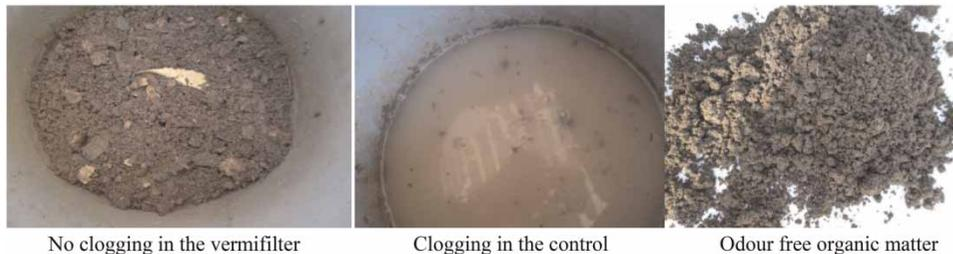
**Figure 4** | Conditions in the vermifilter and control.
