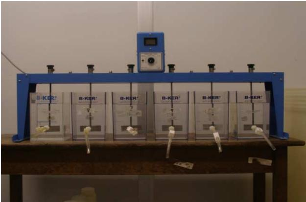
Figure 1 | Jar test set up.
