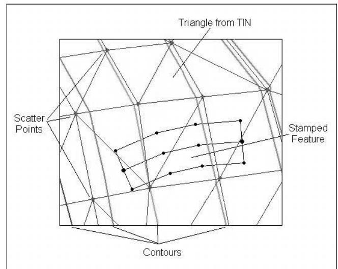
**Figure 9** | TIN with contours under stamped feature.
