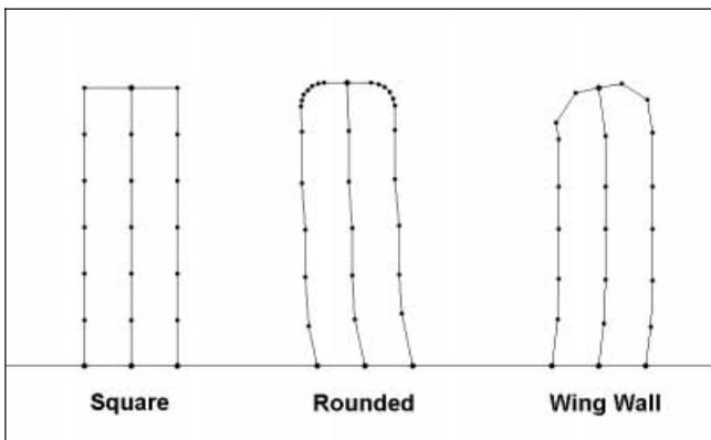
**Figure 8** | Vertical walled embankment end modifications.
