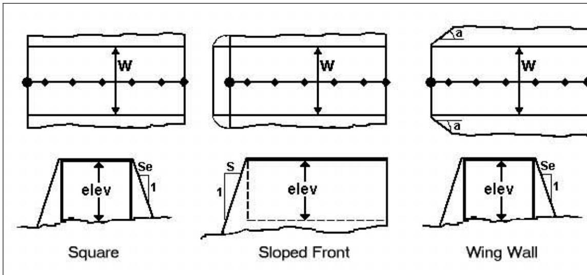
**Figure 4** | Sloped wall end types. The variables  $Se$ ,  $S$  and  $a$  represent the side slope run per unit rise, the end slope run per unit rise and the angle of the wing wall. Other variables are the same as in Figure 3.
