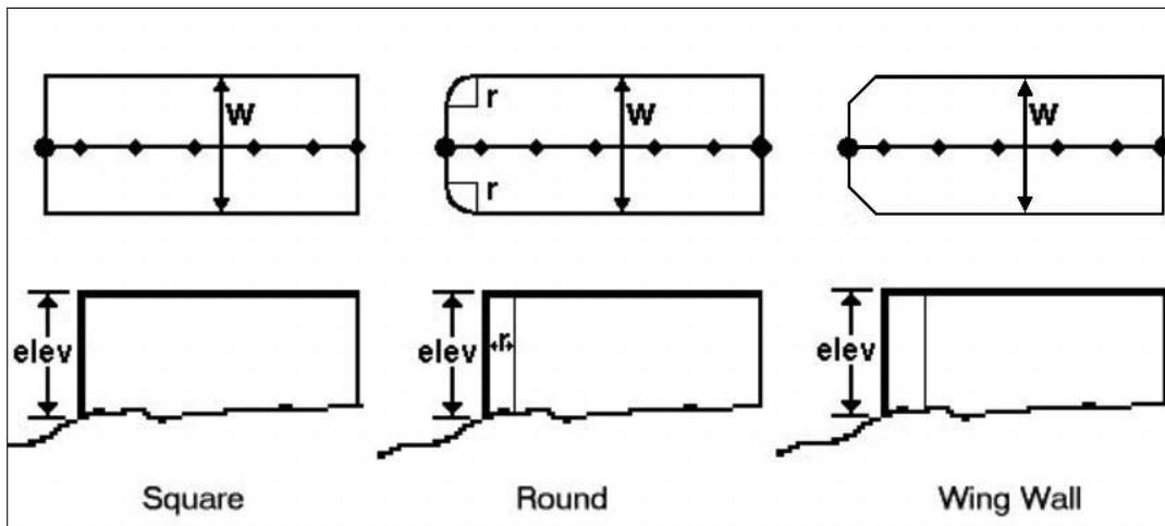
**Figure 3** | Vertical wall end types—side and top views. The variables  $W$ ,  $r$  and  $elev$  represent the width of the flat zone (i.e. the width of the top of the embankment), the radius of curvature, and the elevation of the flat zone relative to a fixed datum, respectively.
