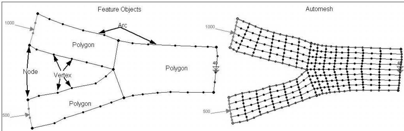
Figure 1 | Sample conceptual model and automatic mesh.
