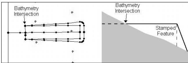
Figure 12 | Intersection of bathymetry and flat zone.
