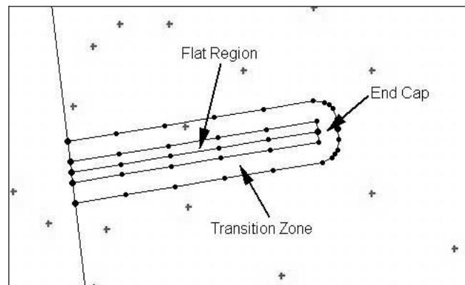
Figure 2 | The parts of a stamped feature.
