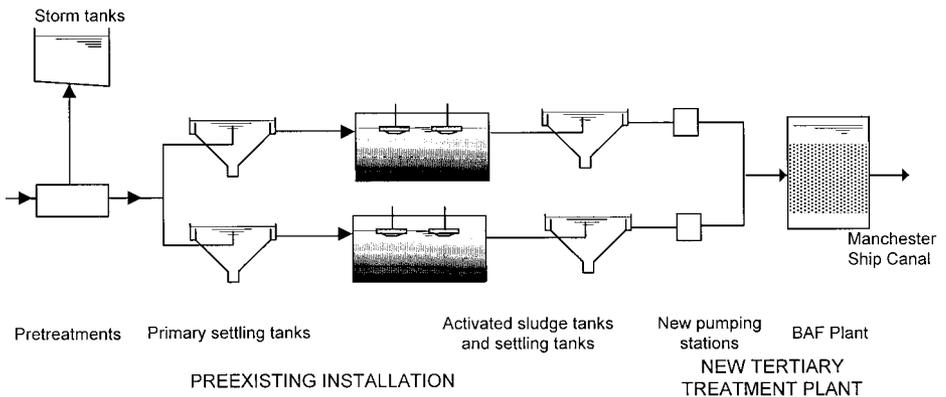
**Figure 1** Davyhulme plant schematic
