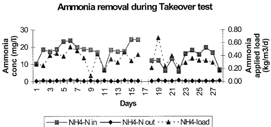
Figure 4 Ammonia removal during take-over test
