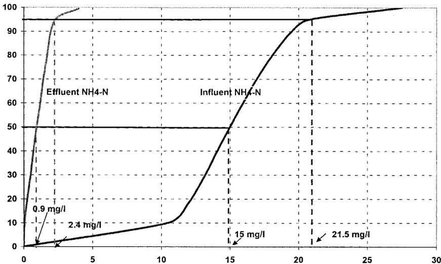
Figure 3 Frequency distribution of the inlet and outlet NH<sub>4</sub>-N concentration
