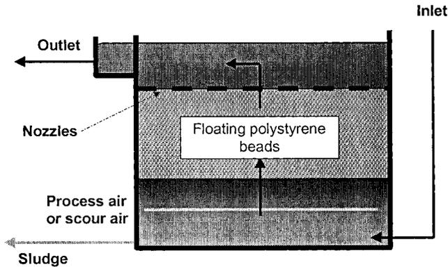
Figure 2 Biostyr process - principle
