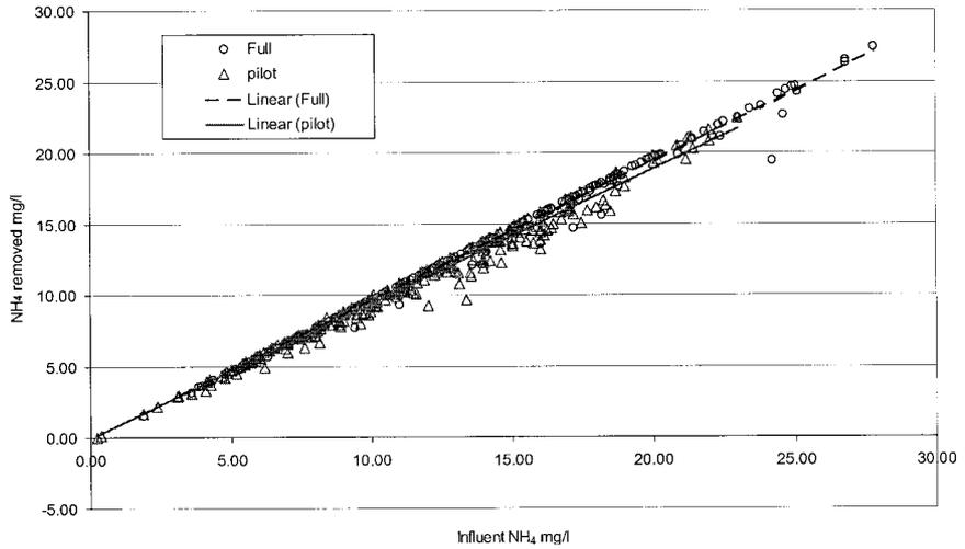
**Figure 6** Comparison between the pilot and the full scale plant.
