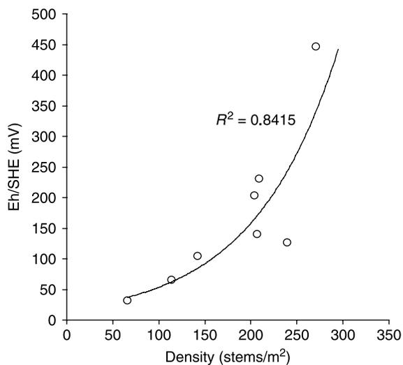
**Figure 7** | Correlation between reed density and redox potential of the sludge deposits for pilots fed with septage with a compost filtration layer and during the second growing season.
