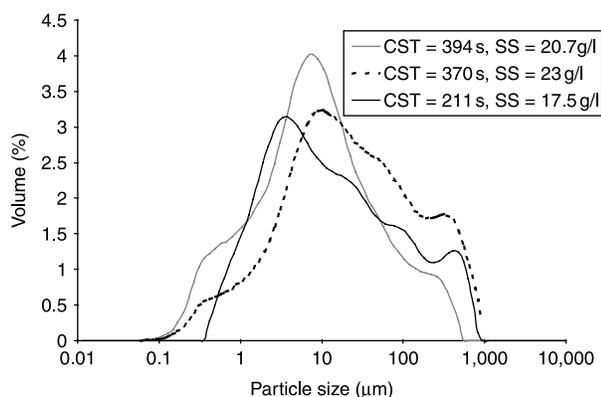
**Figure 5** | Three septage particle size distributions in volume obtained by means of a laser granulometer (Malvern Mastersizer).
