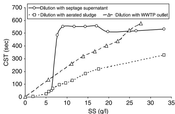
**Figure 1** | Sludge dewaterability (CST) at different suspended solids concentration obtained with septage supernatant, WWTP outlet, or with aerated sludge dilutions.
