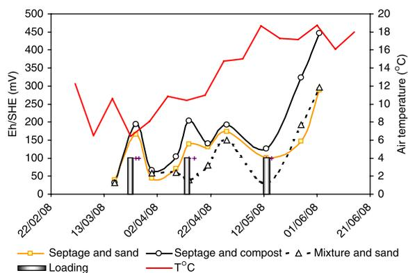
**Figure 6** | Redox potential variations in residual sludge in the experimental beds fed with septage or mixture.
