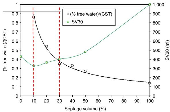
**Figure 2** | Dewaterability and settled volume after 30 min in a 1 liter test tube (SV30) at different septage/aerated sludge volume ratio ( $[\text{SS}]_{\text{septage}} = 26.3 \text{ g/l}$ ,  $[\text{SS}]_{\text{aerated sludge}} = 1.6 \text{ g/l}$ ).
