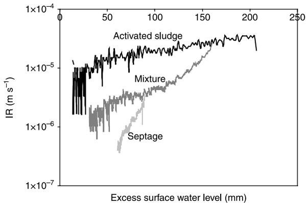
**Figure 8** | Variations of the infiltration rates (IR) for 3 different sludges at a same solid load in pilots with a sand filtration layer and at the second day of feeding.
