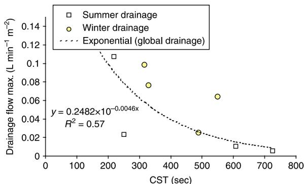
**Figure 9** | Maximum outflow on pilots fed with septage the first day of the loading cycle following the CST.
