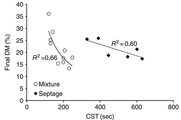
**Figure 10** | Final DM content of the sludge deposit at the end of the rest period in winter ( $9 \pm 5^\circ\text{C}$ ) vs CST of the applied sludge.
